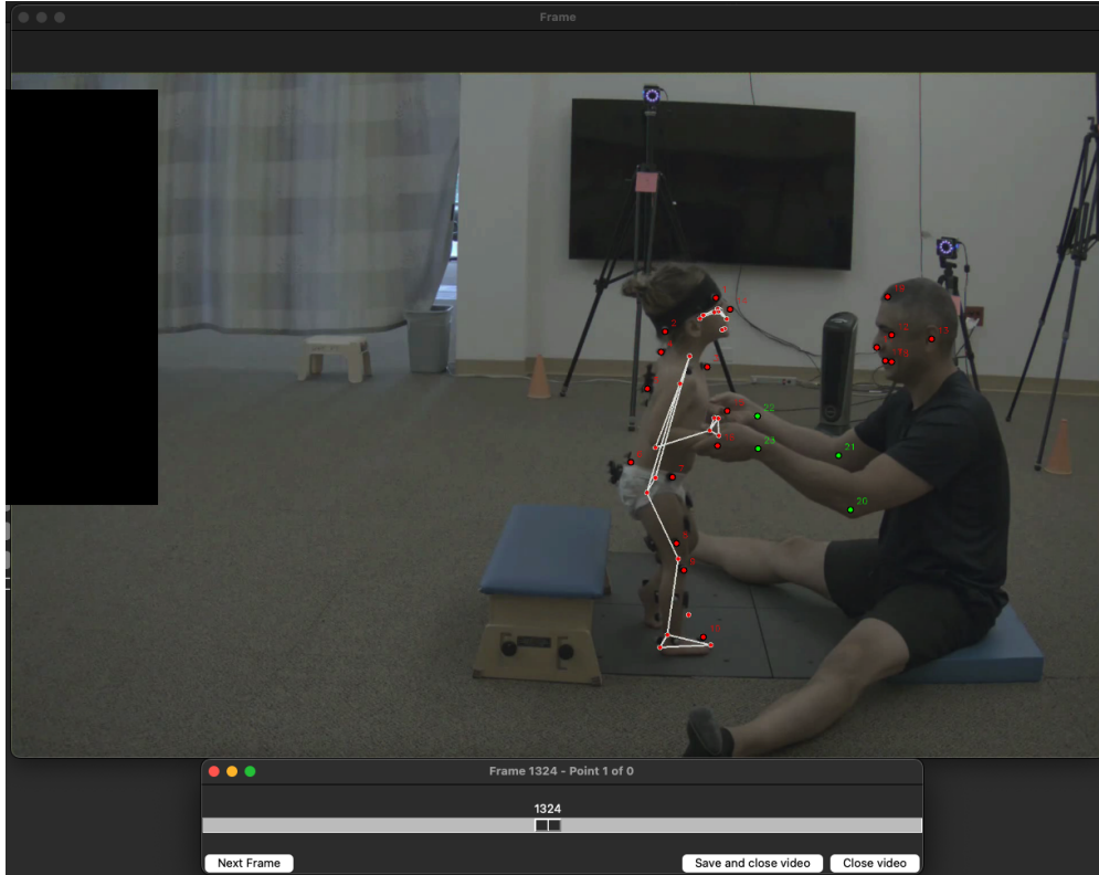
Figure 3: Screenshot of the Get Pixel Coordinate tool within vailá . The interface allows users to navigate video frames, zoom in for precise point selection, and mark or adjust keypoints. This tool facilitates manual annotation and verification of keypoints in video data, enhancing the flexibility of the vailá toolbox.
